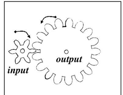
A ratio can be used to show the gain in torque: it is known as mechanical advantage, and it is the reciprocal of the velocity ratio.
