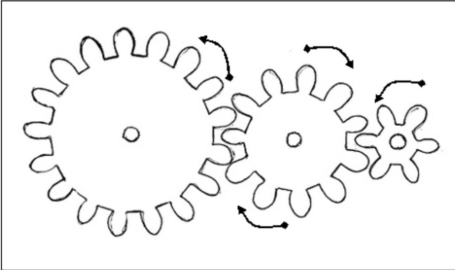
In the above, although we restore the counter clockwise motion of the large small gear, introducing the middle gear does not change the overall gear ratio. Specifically if we hooked up
