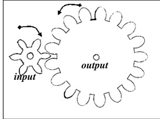
So in the above diagram, if the power is applied to the small wheel, the gear ratio will be 6 to 17 or 6/17. Since the fraction is less than 1 it implies that there will be a loss in velocity. If we apply the turning force to the larger gear, the ratio will be the reciprocal: 17/6, and the output gear will experience a gain in velocity.
